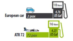
On a 200 Nm sector, the ATR 72-600 fuel consumption per passenger is up to 11% lower than a typical European car.
