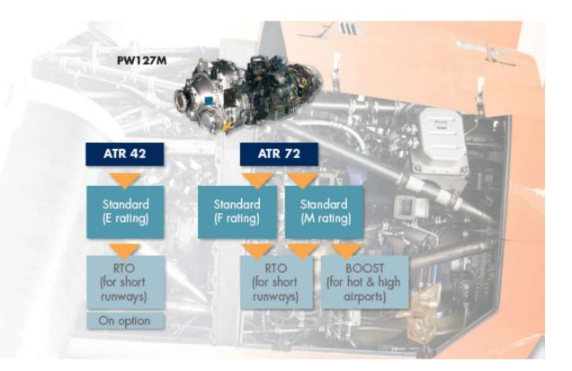
Engine rating selected through airframe identification system (EECR Electronic Engine Control Rating). Through the 'Flex Operation' concept, two levels of power are available for ATR72, allowing either PW127F ratings for standard operations or PW127M for 'Hot & High' operations
